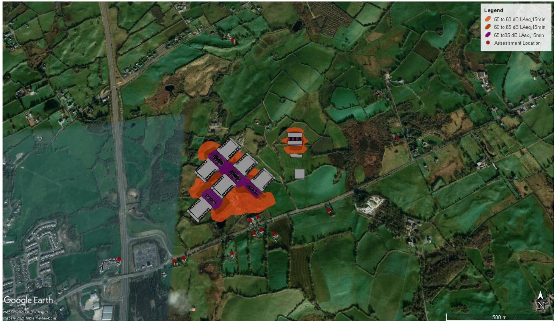
**Figure 9.7** Scenario B Proposed Data Storage Facility (current planning application) – Emergency Noise Contour (Extent of 55dB(A) noise contour)
